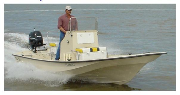
Modified Cathedral hull design provides smooth dry ride. Pocket tunnel allows shallow water operation. Fiberglass composite construction. Custom deck layouts. 7 ft 5 in Beam
