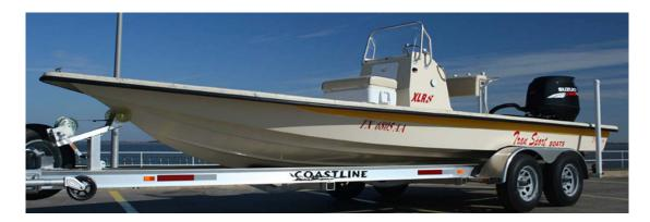
The LS is the low side edition of the XLR8. It is a modified Vee hull with step tunnel and keel pad. This wide beam, quick to plane hull is fast and fuel efficient. The boat is stable at rest and tracks extremely well at speed. The ride is dry and smooth with storage in bow, stern and console compartments. Custom deck layouts. Construction is fiberglass composite.
