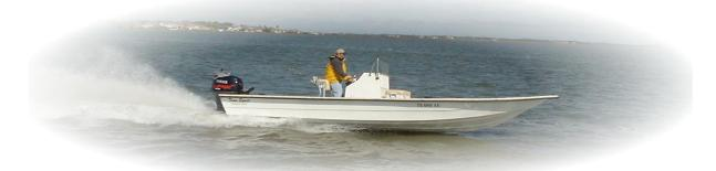
The newest addition to the popular Tran Fiberglass Boat line, the XLR8 is a modified Vee hull with step tunnel and keel pad. This wide beam, quick to plane hull is fast and fuel efficient. The boat is stable at rest and tracks extremely well at speed. The ride is dry and smooth with ample storage in bow, stern and console compartments. Custom deck layouts allow you to configure the design of the boat to fit your needs and desires. Construction is fiberglass composite.
